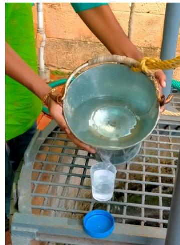
Fig: Filling the sample
